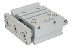
Metal Work pneumatic cylinder, dual guide rod, 40mm bore, 16mm rod diameter, 50mm stroke, double acting, magnetic piston, universal mount.
