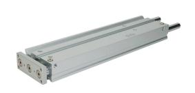
Metal Work pneumatic cylinder, dual guide rod, 32mm bore, 16mm rod diameter, 400mm stroke, double acting, magnetic piston, universal mount.
