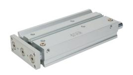
Metal Work pneumatic cylinder, dual guide rod, 32mm bore, 16mm rod diameter, 200mm stroke, double acting, magnetic piston, universal mount.
