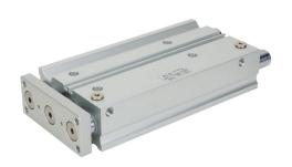
Metal Work pneumatic cylinder, dual guide rod, 32mm bore, 16mm rod diameter, 175mm stroke, double acting, magnetic piston, universal mount.
