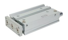
Metal Work pneumatic cylinder, dual guide rod, 32mm bore, 16mm rod diameter, 150mm stroke, double acting, magnetic piston, universal mount.
