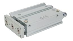
Metal Work pneumatic cylinder, dual guide rod, 32mm bore, 16mm rod diameter, 125mm stroke, double acting, magnetic piston, universal mount.
