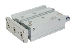
Metal Work pneumatic cylinder, dual guide rod, 32mm bore, 16mm rod diameter, 100mm stroke, double acting, magnetic piston, universal mount.
