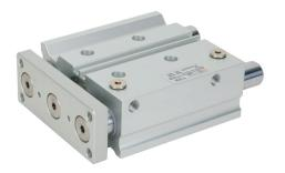
Metal Work pneumatic cylinder, dual guide rod, 32mm bore, 16mm rod diameter, 75mm stroke, double acting, magnetic piston, universal mount.
