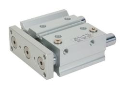
Metal Work pneumatic cylinder, dual guide rod, 32mm bore, 16mm rod diameter, 50mm stroke, double acting, magnetic piston, universal mount.
