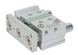
Metal Work pneumatic cylinder, dual guide rod, 32mm bore, 16mm rod diameter, 25mm stroke, double acting, magnetic piston, universal mount.
