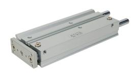
Metal Work pneumatic cylinder, dual guide rod, 25mm bore, 12mm rod diameter, 200mm stroke, double acting, magnetic piston, universal mount.
