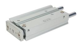
Metal Work pneumatic cylinder, dual guide rod, 25mm bore, 12mm rod diameter, 175mm stroke, double acting, magnetic piston, universal mount.
