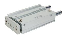
Metal Work pneumatic cylinder, dual guide rod, 25mm bore, 12mm rod diameter, 125mm stroke, double acting, magnetic piston, universal mount.
