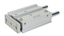
Metal Work pneumatic cylinder, dual guide rod, 25mm bore, 12mm rod diameter, 100mm stroke, double acting, magnetic piston, universal mount.
