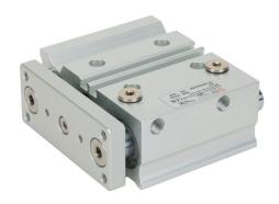
Metal Work pneumatic cylinder, dual guide rod, 25mm bore, 12mm rod diameter, 40mm stroke, double acting, magnetic piston, universal mount.
