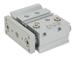
Metal Work pneumatic cylinder, dual guide rod, 25mm bore, 12mm rod diameter, 30mm stroke, double acting, magnetic piston, universal mount.
