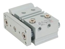
Metal Work pneumatic cylinder, dual guide rod, 25mm bore, 12mm rod diameter, 20mm stroke, double acting, magnetic piston, universal mount.
