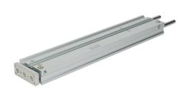
Metal Work pneumatic cylinder, dual guide rod, 20mm bore, 10mm rod diameter, 400mm stroke, double acting, magnetic piston, universal mount.
