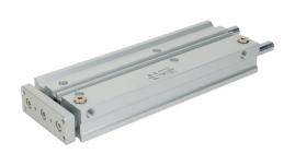
Metal Work pneumatic cylinder, dual guide rod, 20mm bore, 10mm rod diameter, 200mm stroke, double acting, magnetic piston, universal mount.
