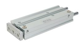
Metal Work pneumatic cylinder, dual guide rod, 20mm bore, 10mm rod diameter, 175mm stroke, double acting, magnetic piston, universal mount.
