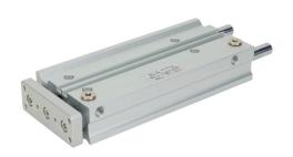
Metal Work pneumatic cylinder, dual guide rod, 20mm bore, 10mm rod diameter, 150mm stroke, double acting, magnetic piston, universal mount.
