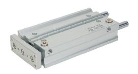
Metal Work pneumatic cylinder, dual guide rod, 20mm bore, 10mm rod diameter, 125mm stroke, double acting, magnetic piston, universal mount.
