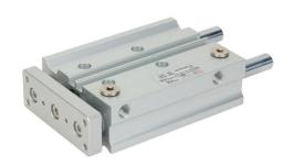
Metal Work pneumatic cylinder, dual guide rod, 20mm bore, 10mm rod diameter, 75mm stroke, double acting, magnetic piston, universal mount.
