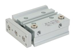
Metal Work pneumatic cylinder, dual guide rod, 20mm bore, 10mm rod diameter, 50mm stroke, double acting, magnetic piston, universal mount.
