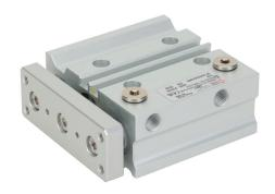
Metal Work pneumatic cylinder, dual guide rod, 20mm bore, 10mm rod diameter, 40mm stroke, double acting, magnetic piston, universal mount.
