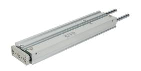
Metal Work pneumatic cylinder, dual guide rod, 16mm bore, 8mm rod diameter, 250mm stroke, double acting, magnetic piston, universal mount.
