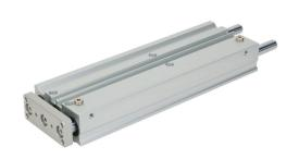
Metal Work pneumatic cylinder, dual guide rod, 16mm bore, 8mm rod diameter, 175mm stroke, double acting, magnetic piston, universal mount.
