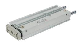
Metal Work pneumatic cylinder, dual guide rod, 16mm bore, 8mm rod diameter, 150mm stroke, double acting, magnetic piston, universal mount.
