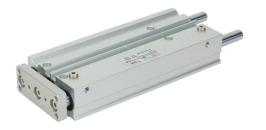
Metal Work pneumatic cylinder, dual guide rod, 16mm bore, 8mm rod diameter, 125mm stroke, double acting, magnetic piston, universal mount.
