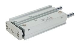
Metal Work pneumatic cylinder, dual guide rod, 16mm bore, 8mm rod diameter, 100mm stroke, double acting, magnetic piston, universal mount.
