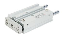
Metal Work pneumatic cylinder, dual guide rod, 16mm bore, 8mm rod diameter, 75mm stroke, double acting, magnetic piston, universal mount.
