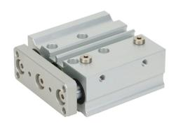
Metal Work pneumatic cylinder, dual guide rod, 16mm bore, 8mm rod diameter, 30mm stroke, double acting, magnetic piston, universal mount.
