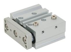
Metal Work pneumatic cylinder, dual guide rod, 16mm bore, 8mm rod diameter, 20mm stroke, double acting, magnetic piston, universal mount.
