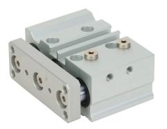
Metal Work pneumatic cylinder, dual guide rod, 16mm bore, 8mm rod diameter, 10mm stroke, double acting, magnetic piston, universal mount.
