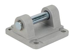
Metal Work rear clevis mount, aluminum. For use with 100mm bore ISO 15552 cylinders. Mounting hardware included.
