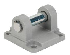
Metal Work rear clevis mount, aluminum. For use with 63mm bore ISO 15552 cylinders. Mounting hardware included.
