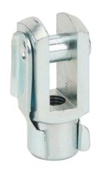
Metal Work rod clevis, M10 X 1.25 thread, plated steel. For use with 25mm bore ISO 6432 cylinders.
