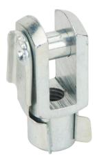
Metal Work rod clevis, M6 x 1.0 thread, plated steel. For use with 12mm and 16mm bore ISO 6432 cylinders.
