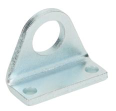
Metal Work foot mount bracket, plated steel. For use with 12mm and 16mm bore ISO 6432 cylinders.
