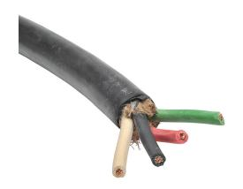
Southwire portable cord, unshielded, W, 2000V, 4 conductors (includes ground), 8 AWG, EPDM thermoset rubber conductor insulation material, black, white, red and green, CPE thermoset rubber jacket, black, cut to length.
