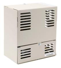
AutomationDirect VTF series drive output filter, 208-600 VAC, 20hp at 460 VAC and 25hp at 575 VAC, UL Type 1, 3-phase, 27A, output side only. For use with multiple AC drives.
