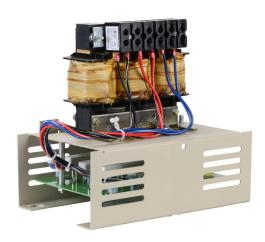
AutomationDirect VTF series drive output filter, 208-600 VAC, 5hp at 208 VAC, 10hp at 460 VAC and 15hp at 575 VAC, 3-phase, 18A, output side only. For use with multiple AC drives.
