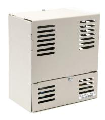
AutomationDirect VTF series drive output filter, 208-600 VAC, 5hp at 208 VAC, 10hp at 460 VAC and 15hp at 575 VAC, UL Type 1, 3-phase, 18A, output side only. For use with multiple AC drives.
