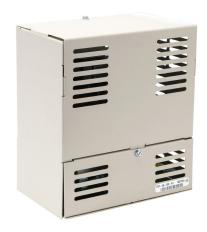
AutomationDirect VTF series drive output filter, 208-600 VAC, 5hp at 208 VAC, 10hp at 460 VAC and 15hp at 575 VAC, UL Type 1, 3-phase, 18A, output side only. For use with multiple AC drives.
