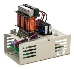
AutomationDirect VTF series drive output filter, 208-600 VAC, 3/4hp at 460 VAC and 1hp at 575 VAC, 3-phase, 2A, output side only. For use with multiple AC drives.
