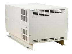
AutomationDirect VTF series drive output filter, 208-600 VAC, 150hp at 230 VAC, 300hp at 460 VAC and 350hp at 575 VAC, UL Type 1, 3-phase, 362A, output side only. For use with multiple AC drives.
