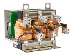
AutomationDirect VTF series drive output filter, 208-600 VAC, 100hp at 230 VAC, 200hp at 460 VAC and 250hp at 575 VAC, open frame, 3-phase, 250A, output side only. For use with multiple AC drives.
