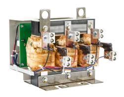
AutomationDirect VTF series drive output filter, 208-600 VAC, 75hp at 230 VAC, 150hp at 460 VAC and 200hp at 575 VAC, open frame, 3-phase, 200A, output side only. For use with multiple AC drives.
