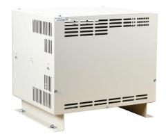
AutomationDirect VTF series drive output filter, 208-600 VAC, 75hp at 230 VAC, 150hp at 460 VAC and 200hp at 575 VAC, UL Type 1, 3-phase, 200A, output side only. For use with multiple AC drives.
