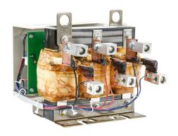
AutomationDirect VTF series drive output filter, 208-600 VAC, 60hp at 230 VAC, 125hp at 460 VAC and 150hp at 575 VAC, open frame, 3-phase, 160A, output side only. For use with multiple AC drives.
