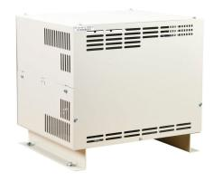
AutomationDirect VTF series drive output filter, 208-600 VAC, 30hp at 208 VAC, 40hp at 230 VAC, 75hp at 460 VAC and 100hp at 575 VAC, UL Type 1, 3-phase, 110A, output side only. For use with multiple AC drives.
